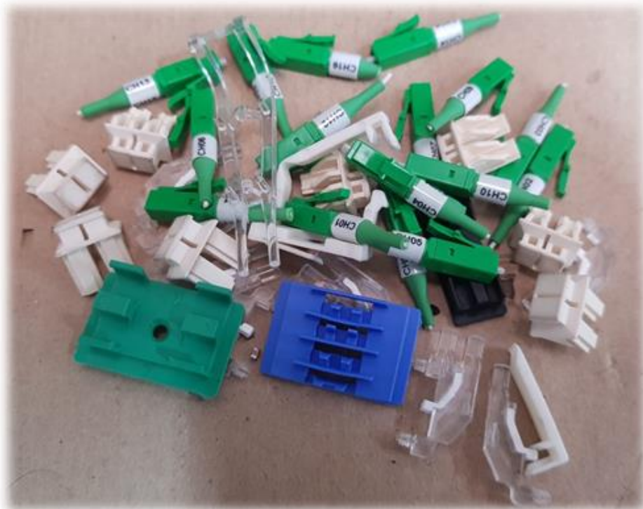
Figure 42. 16ALM plastic parts after disassembly.
