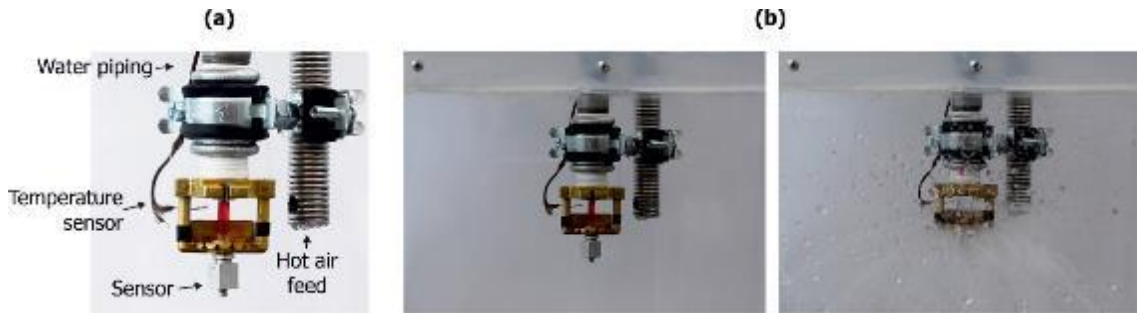
Figure 55. Sprinkler sensor evaluation setup
