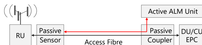
Figure 28. Application of an ALM in radio-access-network monitoring. RU: radio unit. DU: data unit. CU: control unit. EPC: evolved packet core.
