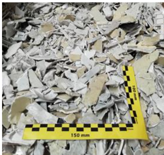
Figure 17. ABS plastic material obtained from WEEE printer parts of other brands
