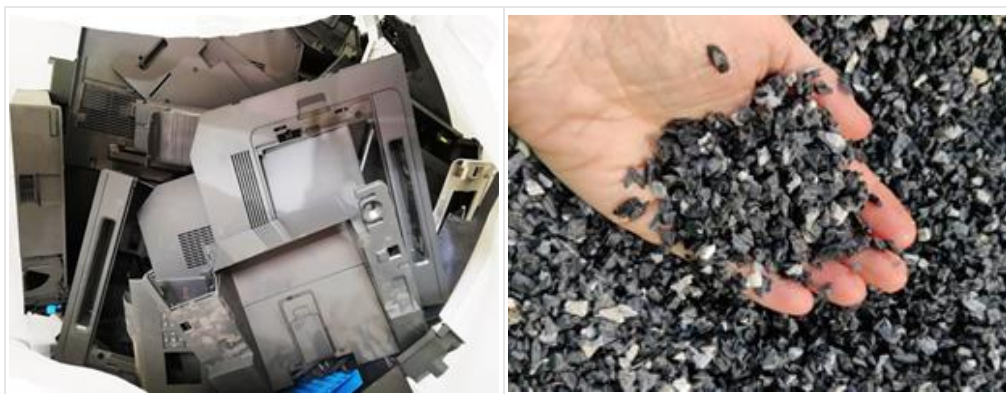
Figure 18. ABS plastic parts from Lexmark printers (left) and ABS flakes obtained after processing (right)
