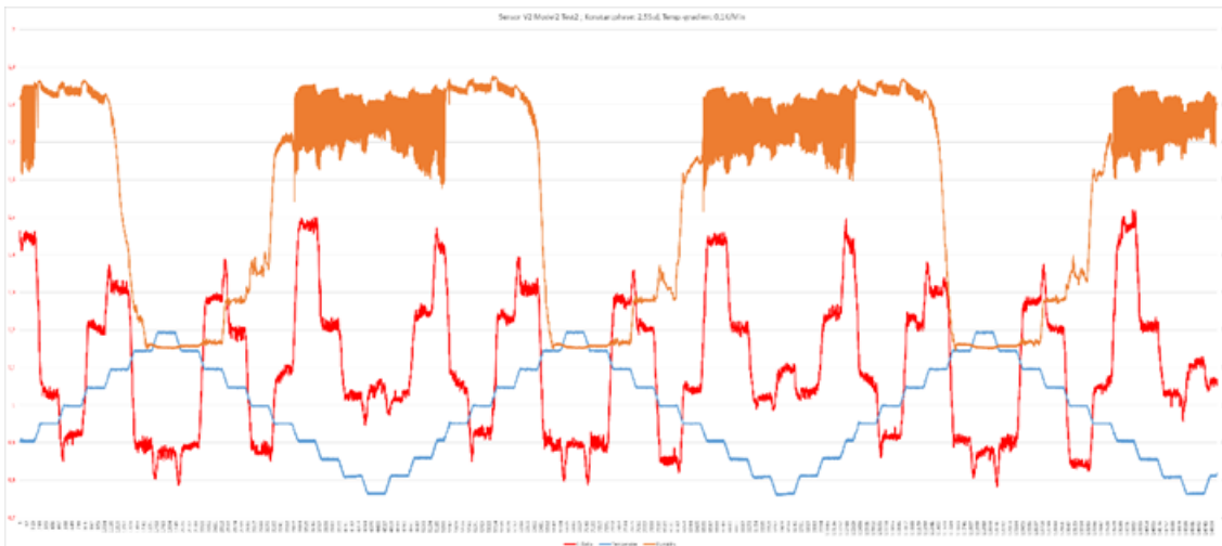
Figure 74. Temperature chamber measurements for the cabinet sensor: Insertion loss (red), humidity (orange) and temperature (blue).
