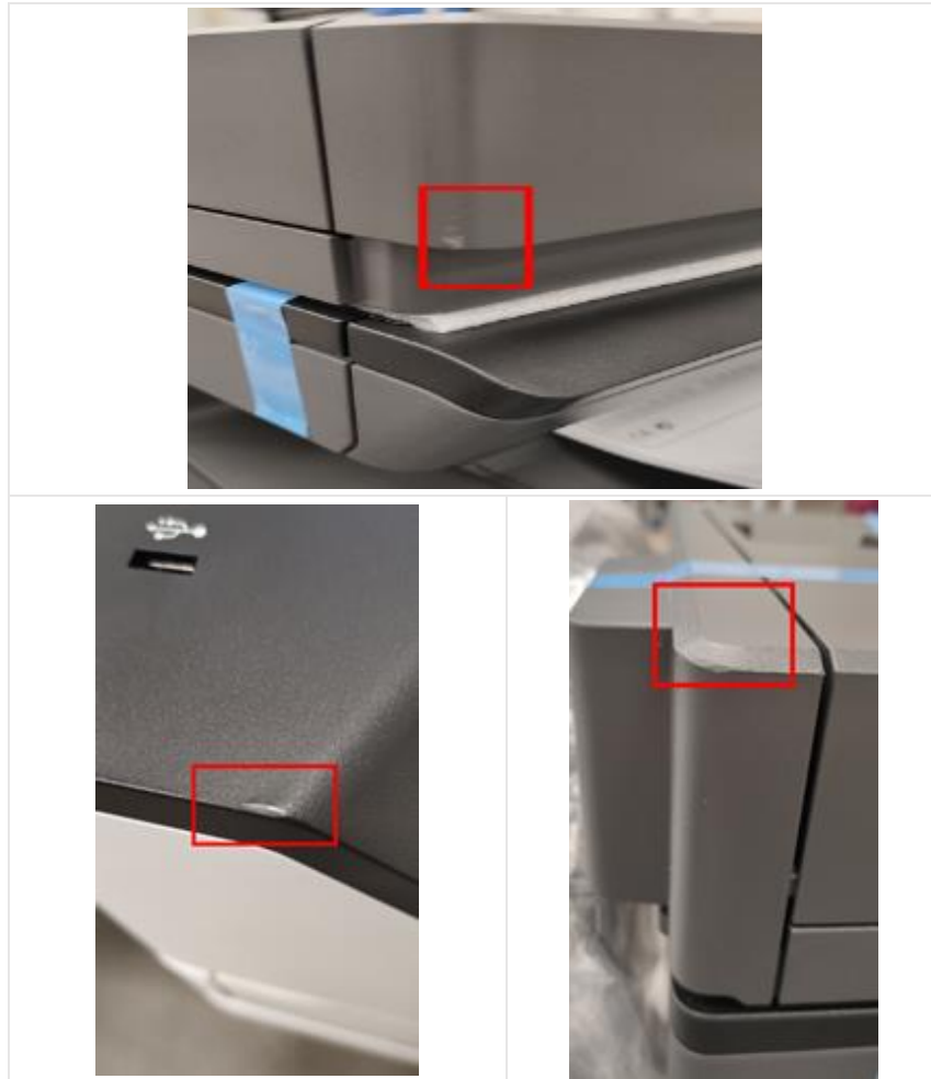
Figure 16. Cosmetic defect samples in refurbished printers
