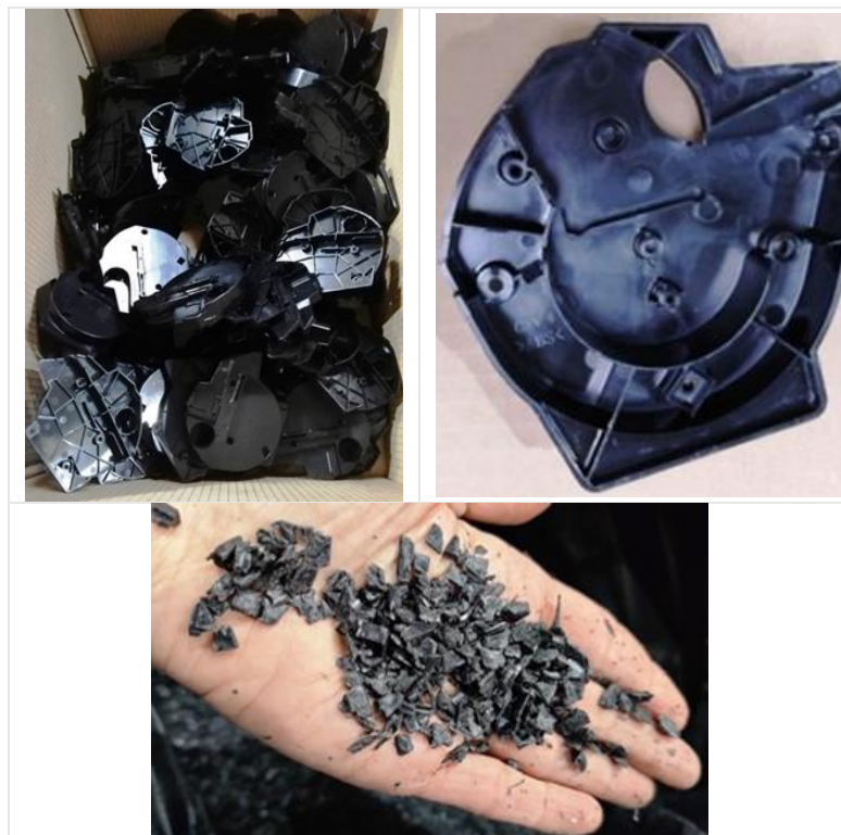
Figure 19. ABS endcaps from Lexmark cartridges (above) and ABS flakes obtained after processing (below)
