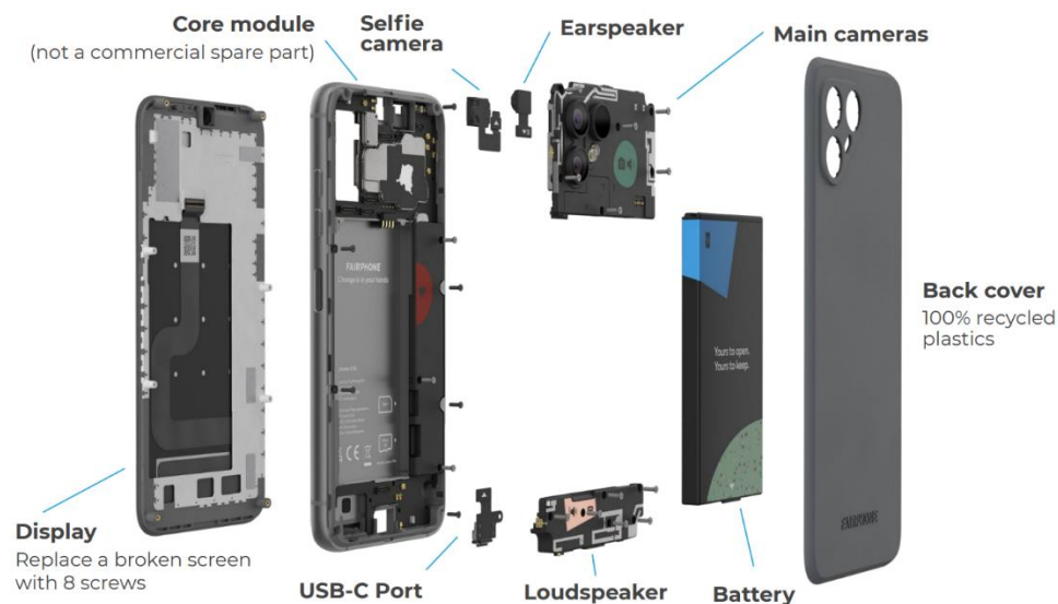
Figure 4.3 – Modular design of Fairphone 4 [17]
