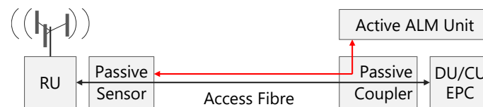
Figure 26. Application of an ALM in radio-access-network monitoring. RU: radio unit. DU: data unit. CU: control unit. EPC: evolved packet core (RU, DU, CU and EPC are part of the Internet).
