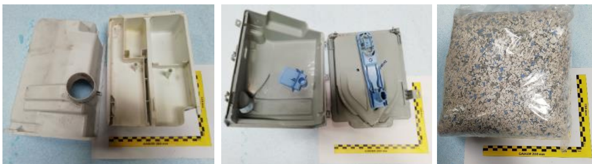
Figure 7. Detergent drawers from EoL washing machines (Beko/Grundig) and PP flakes obtained
