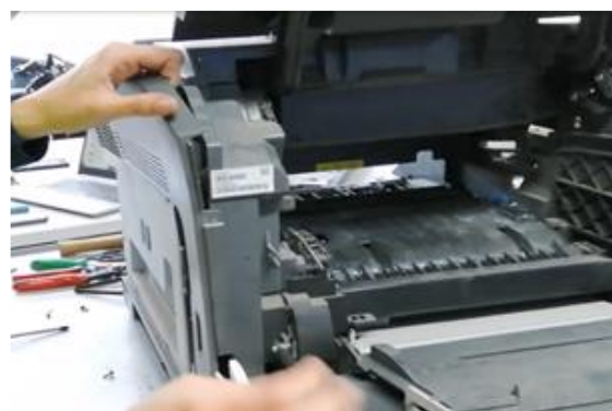
Dismantling of left cover
