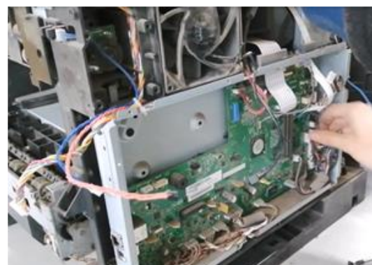
Dismantling of mother board
