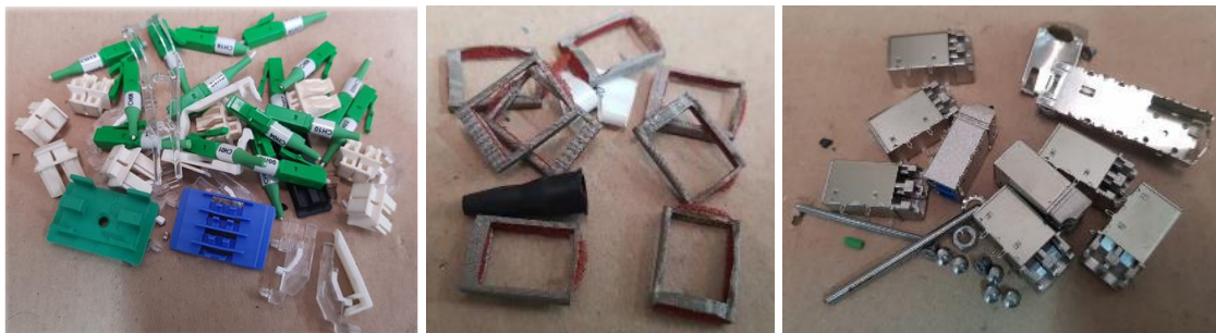
Figure 32. 16ALM plastic parts (left), rubber (centre) and metal (right) after disassembly.
