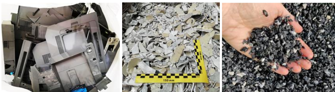
Figure 22. ABS plastic parts from Lexmark printers (left), non-Lexmark printers (center) and ABS flakes obtained after processing (right)
