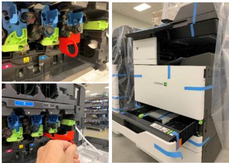
Figure 20. In red, the parts used to lock the cartridges (left) and the drawer (right) during transportation
