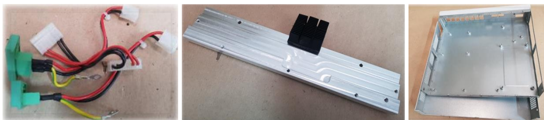
Figure 33. 16ALM cables, Al heat sink and chassis after disassembly.
