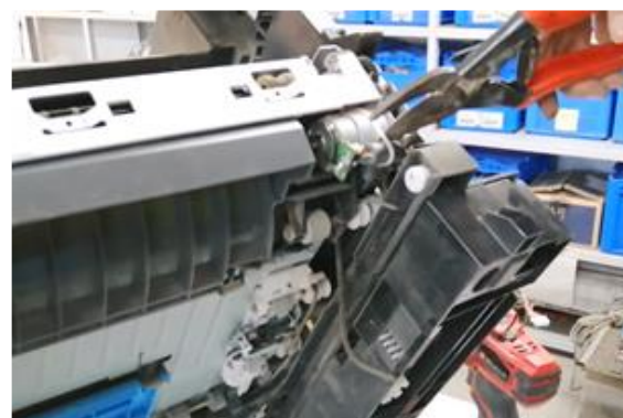
Dismantling of duplex motor with cable
