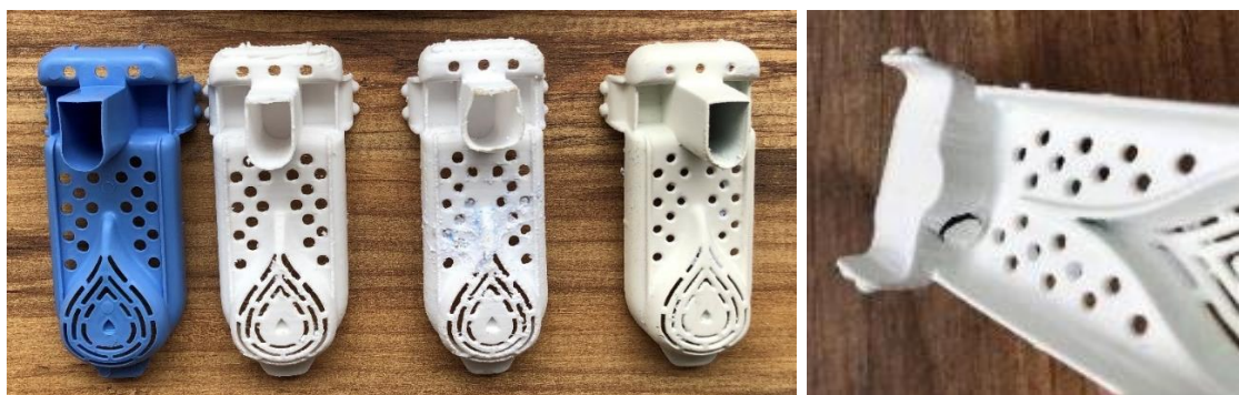
Figure 4. 3D printed siphons, left to right: original liquid detergent siphon, 3D printed siphon, 3D printed siphon after the test, 3D printed and polished siphon, cracked siphon after testing.
