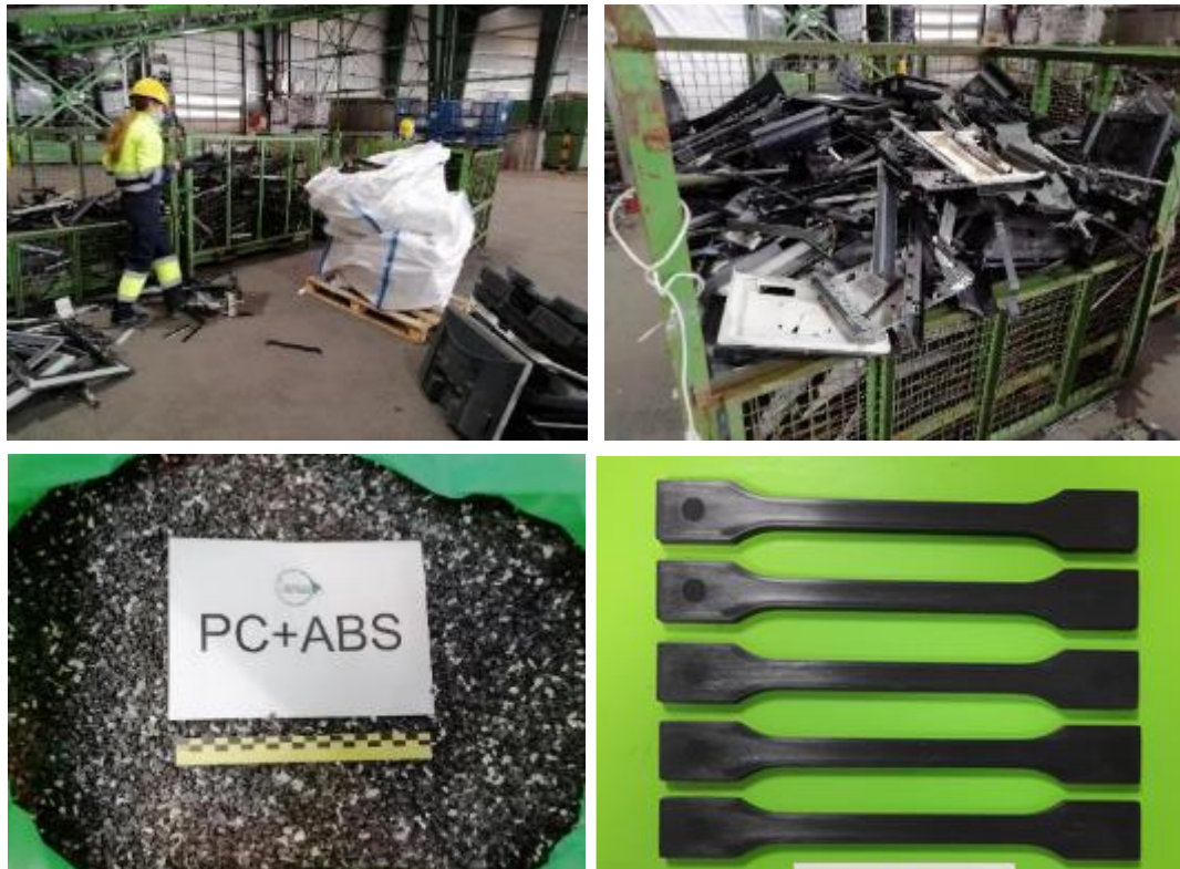
Figure 47. Selection of TV parts at Indumetal for recovery of recycled plastics (above) and material flakes and testing specimens obtained (below)
