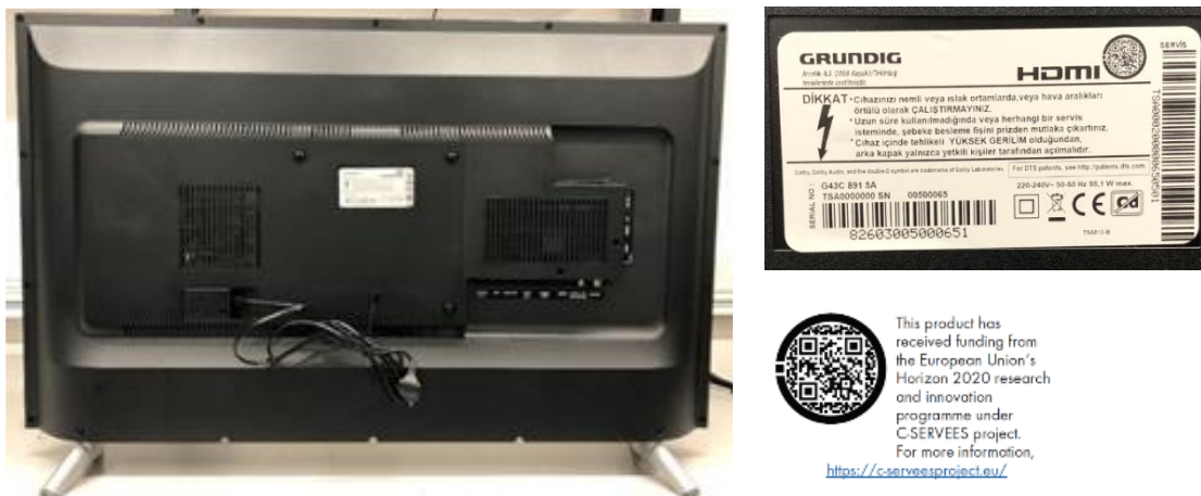
Figure 41. Back TV panel with recycled content and QR code in the demo TVs.
