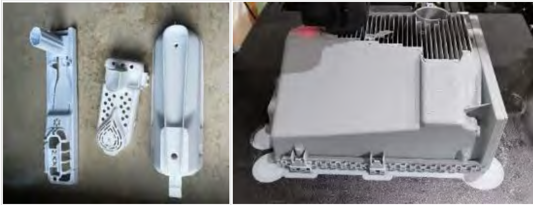
Figure 8. Selected washing machine's suitable parts /components for 3D printing tests
