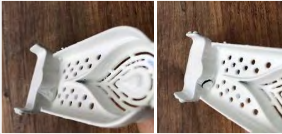
Figure 14. 3D printed and unpolished siphon part surface (swelled and cracked) after testing
