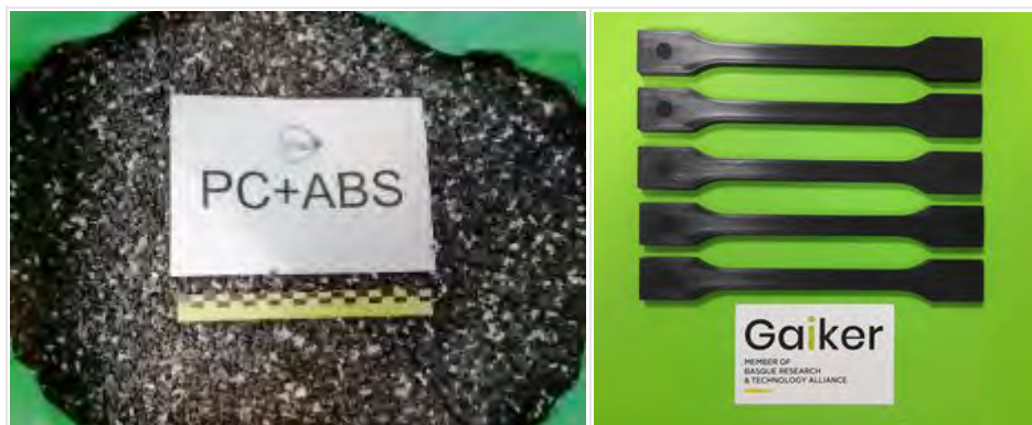
Figure 73. PC-ABS flakes (left) and testing specimens (right)
