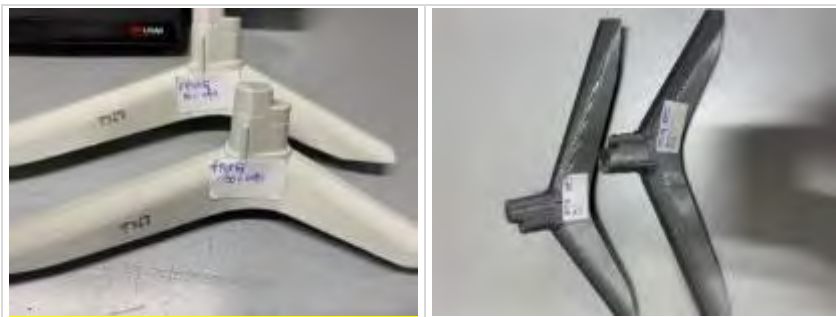
Figure 67. 1.2 FACILAN C8 material, rPETG 30 % infill density (left) and 1.3 PET G material - 20 % infill density and 0.2 layer (right)
