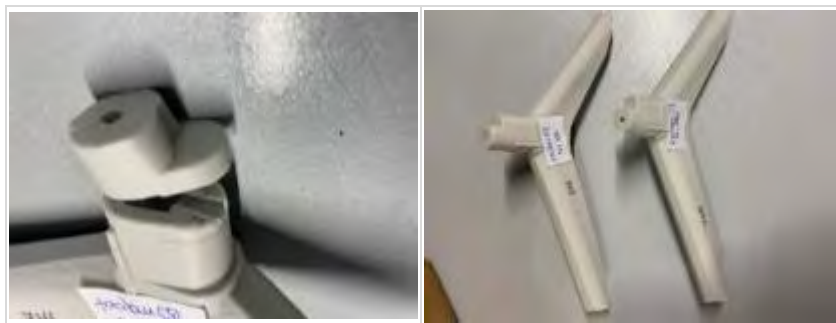
Figure 66. 1.1 FACILAN C8 material, 30 % infill density
