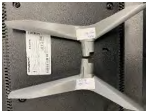
Figure 68. 1.4 PETG material - with the infill density of 30 %, 15% and 20%.
