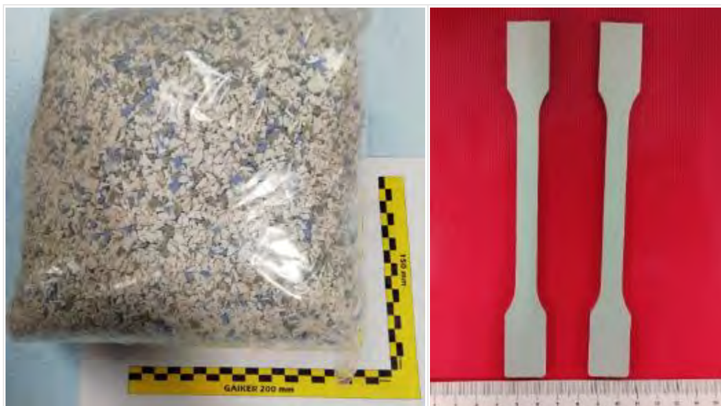
Figure 16. Recycled PP flakes from detergent drawers (left) and injected specimens (right)
