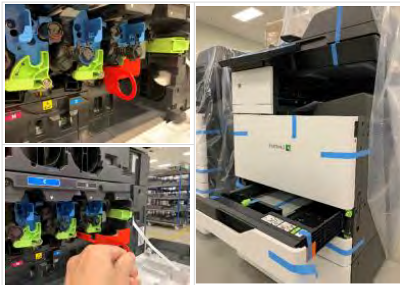
Figure 22. In red, the parts used to lock the cartridges(left) and the drawer (right) during transportation
