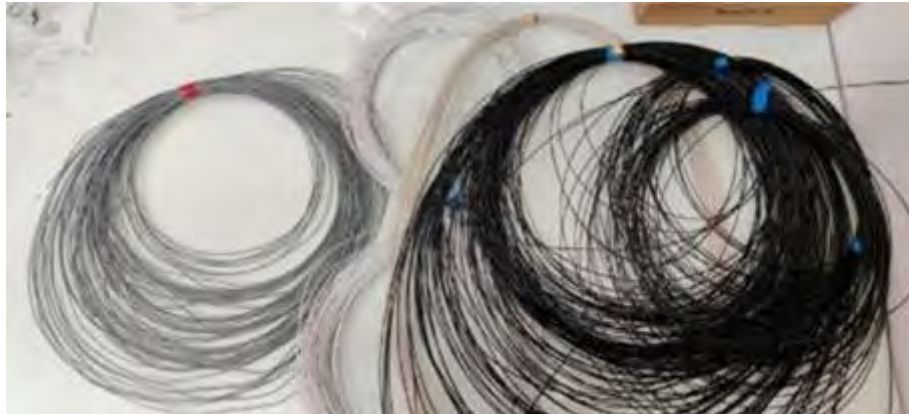
Figure 9. Filaments from extruded polymer pellets to use in WM 3D printing tests
