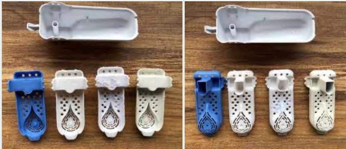
Figure 12. Liquid detergent container group, front face (left) and rear face (right). Upper side: liquid detergent container cover. Lower side, left to right: original liquid detergent siphon, 3D printed liquid detergent siphon, 3D printed liquid detergent siphon after the test, 3D printed and polished liquid detergent siphon
