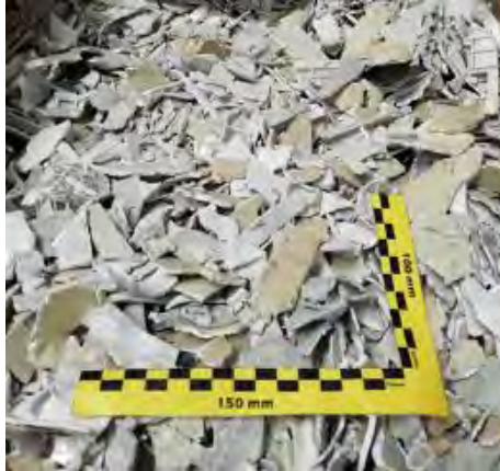
Figure 20. Sample of shredded printer parts (ABS only) from Greentronics
