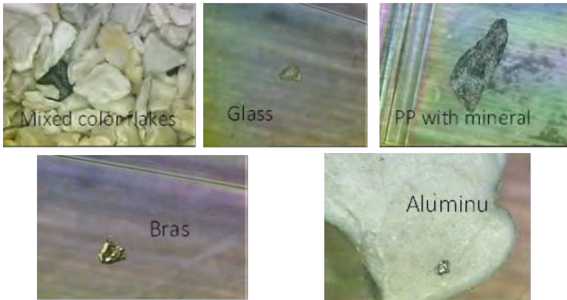
Figure 21. Samples of particles found in the ABS sample analysed at Lexmark
