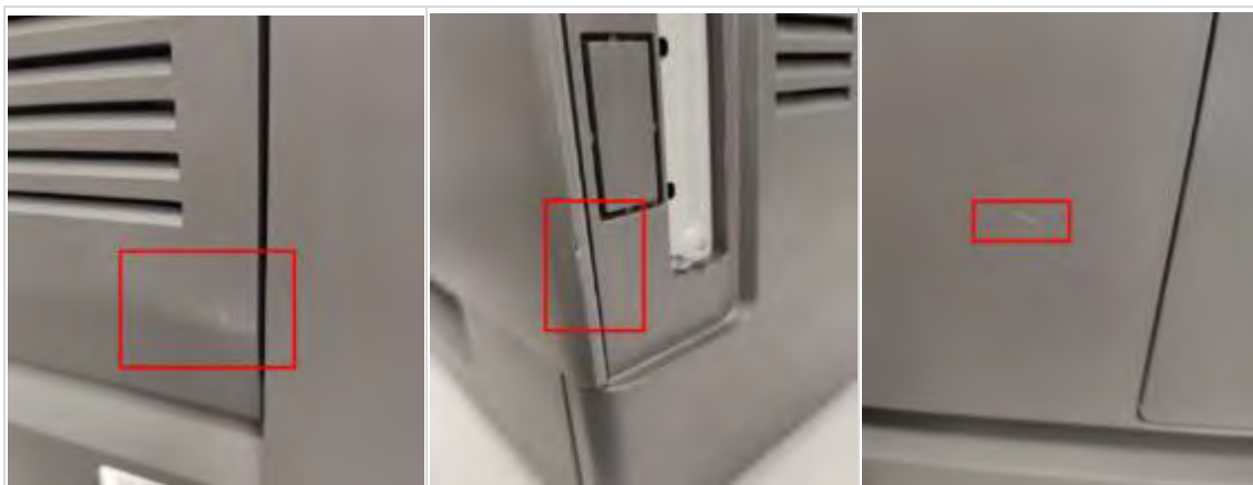
Figure 25. Cosmetic defect samples on housings used for the activity
