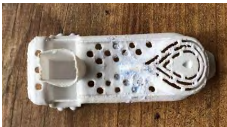
Figure 13. 3D printed and unpolished siphon part surface after testing
